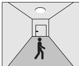
With sufficient daylight, (>300Lux) even when motion detected, light remains off.
