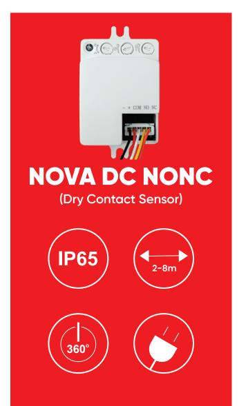
The sensor is an active motion detector, it emits high-frequency electro-magnetic wave (5.8GHz) and receives their echo. The sensor detects the change in echo from even the slightest movement in its detection zone. A microprocessor then triggers the "switch light ON" command. Detection is possible through doors, panes of glass or thin walls.
