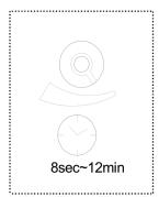
1) Time Setting: The light can be set to stay ON for any period of time between approx. 8sec (turn fully anti-clockwise) and a maximum of 12min (turn fully clockwise). Any movement detected before this time elapse will re-start the timer. It is recommended to select the shortest time for adjusting the detection zone and for performing the walk test.
