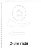
1) **Reach setting (sensitivity):** Reach is the term used to describe the radius of the circular detection zone produced on the ground. After mounting the sensor light at a height of 2.5m, turn the reach control completely in anti-clockwisedirection to select minimum reach (approx.2 m radius), and turn the reach control completely in a clockwise direction to select the maximum reach (approx. 8m radius).
