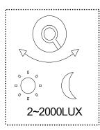
2) Light Control Setting: The chosen light response threshold can be infinitely from approx. 2-2000lux. Turn it fully anti-clockwise to select dusk- to-dawn operation at about 2 Lux. Turn it fully clockwise to select daylight operation at about 2000lux. The knob must be turned fully clockwise when adjusting the detection zone and performing the walk test in daylight.
